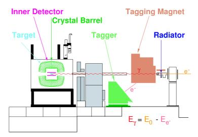
FIGURE 1. Setup of the CB-ELSA detector for a first series of measurements
