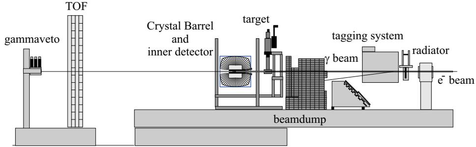
**FIGURE 1.** Experimental setup: Initial configuration of the CB-ELSA experiment
