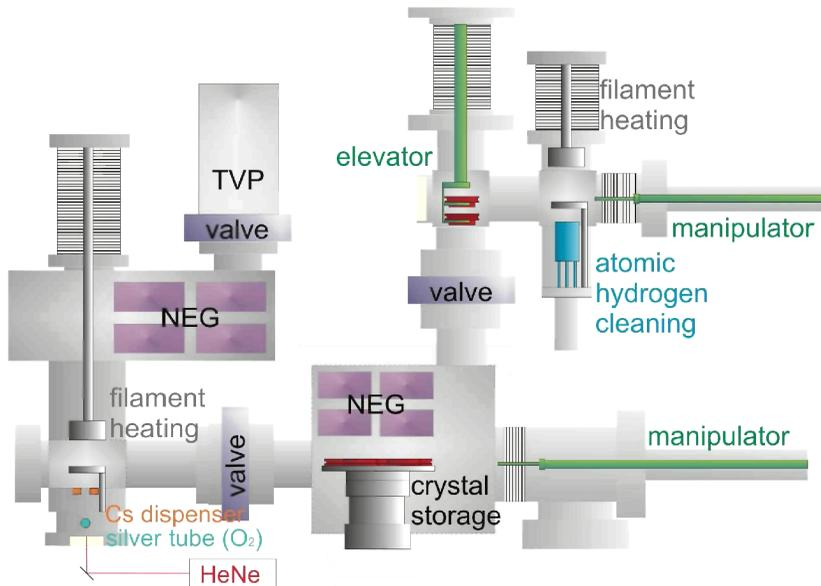
FIGURE 5. New load-lock with crystal storage and atomic hydrogen cleaning.
