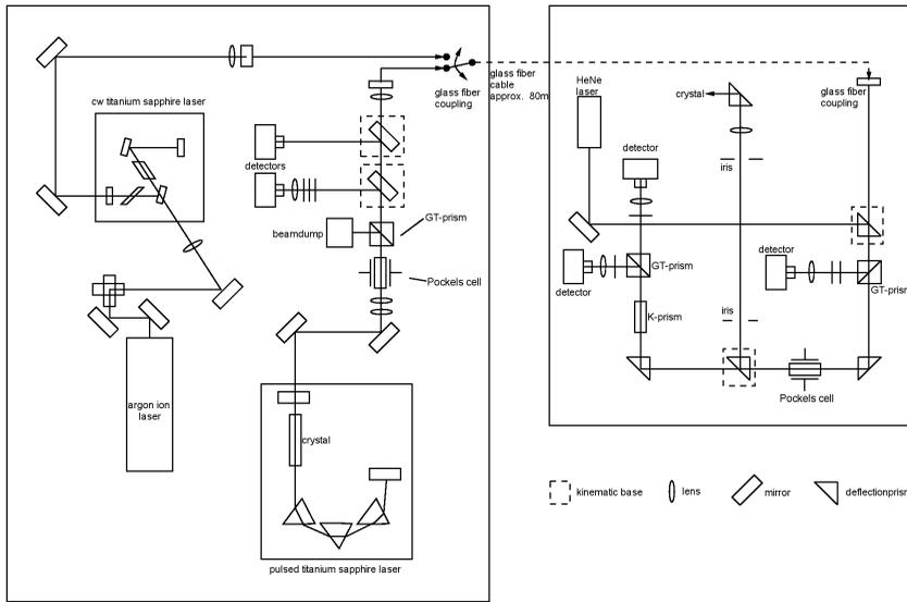
**FIGURE 3.** Optical tables in the laser room (left) and under the 50 keV source (right).
