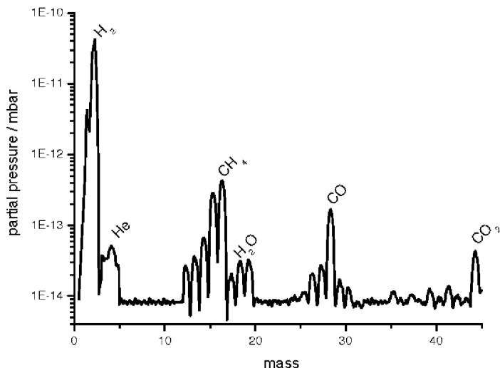
FIGURE 2. Partial pressures of various gas species in the gun chamber.
