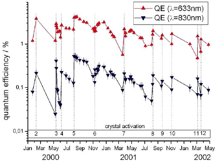
FIGURE 4. Overall degradation of the quantum efficiency.
