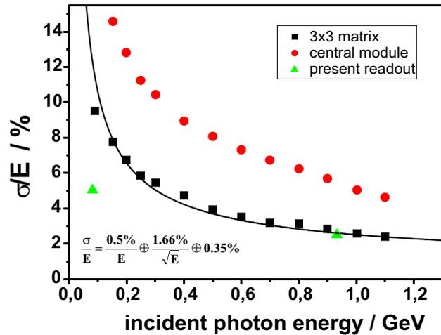
**Figure 7.** Energy resolution with the APD readout, compared to the current PD readout.
