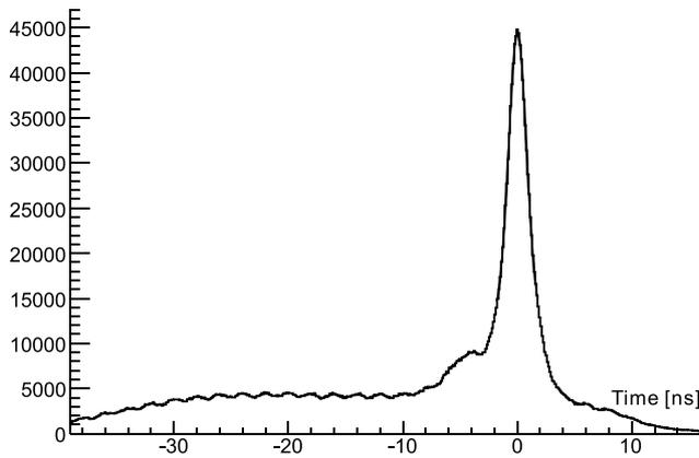
**Figure 4.** Calibrated time resolution for photons in the Forward Detector CsI(Tl) calorimeter. With a  $\sigma(t)$  of 1.3 ns, the detector is able to resolve the bunch structure of the accelerator
