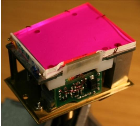
**Figure 8.** Readout option with two  $9\text{ mm}^2$  SiPMs additionally attached to the WLS of the current setup.
