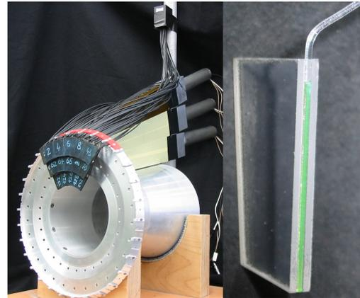
**Figure 9.** New subdetector for charge identification in the Crystal Barrel Forward Detector (left), based on 3 mm plastic scintillators with thermoformed fibre readout (right).
