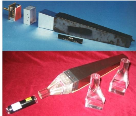
**Figure 3.** Photodiode readout of one of the main calorimeter crystals (top) and PMT readout of one of the forward calorimeter crystals (bottom).
