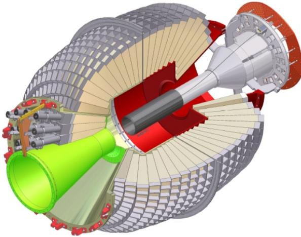
**Figure 2.** The *Crystal Barrel calorimeter* (center) with its *Inner Detector* (from the right) and the *Crystal Barrel Forward Detector* (from the left).
