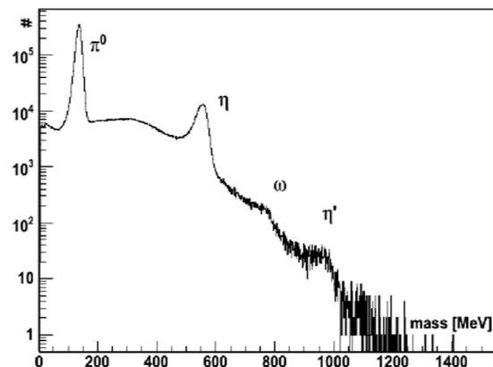
**Figure 5.** Online  $\gamma\gamma$ -invariant mass spectrum for events with three clusters (1 charged + 2 neutral) in the calorimeters.
