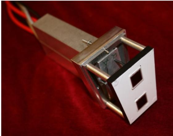
**Figure 6.** Readout option with two 1 cm<sup>2</sup> APDs attached directly to the CsI(Tl) crystals.
